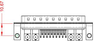
POWER/CO-AX CONTACT RATING: (IF PRESENT) SIGNAL CONTACT CURRENT RATING: 5A PER CONTACT SIGNAL CONTACT RESISTANCE:  $10m\Omega$  MAX.
