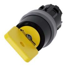
Key-operated switch O.M.R, 22 mm, round, plastic with metal front ring, lock number 73033, yellow, with 2 keys, 2 switch positions O<I, momentary contact type, Actuating angle 45°, 10:30h/12h, key removal O, with laser labeling, upper case and lower case, always upper case at the beginning of the word
