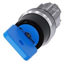
Key-operated switch O.M.R, 22 mm, round, metal, shiny, lock number 73038, blue, with 2 keys, 2 switch positions O-I, latching, actuating angle  $90^{\circ}$ , 10:30h/13:30h, key removal O+I, with laser labeling, upper case
