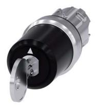
key-operated switch Siemens, 22 mm, round, metal, shiny, lock number SSG10, with 2 keys, 3 switch positions I-O<II, left latching, momentary contact type on the right, actuating angle  $2\times45^{\circ}$ , 10:30h/12h/13:30h, key removal I, with laser labeling, upper case and lower case, always upper case at beginning of line
