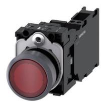
Illuminated pushbutton, 22 mm, round, plastic with metal front ring, red, pushbutton, flat, momentary contact type, with holder, 1 NO+1 NC, LED module with integrated LED 24 V AC/DC, spring-type terminal, Z=20-unit packaging
