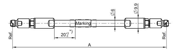
All dimensions are in mm; tolerances:  $\pm$  3mm for A  $\leq$  300 mm;  $\pm$  1% for A > 300 mm \*) If length "A" < 150 mm marking is mount centric  $\pm$ 5 mm
