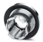
M12 threaded sleeve with tolerance-compensating function, for straight, SMD-solderable M12 socket contact inserts. Suitable for  $0.9 \text{ mm} \dots 1.6 \text{ mm}$  thick front plates.
