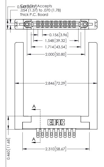
0.295[7.49] Card Slot ECTION 0.090 [2.29] Point of Contact 305 ENG MASTER 305 / 315 / 355 Card Edge Connector J.LEE DATE: SEPT. 21/09 Part Number: 315-018-500-258
