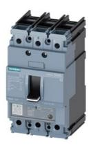
circuit breaker 3VA5 UL frame 125 breaking capacity class M 35kA @ 480 V 3-pole, line protection TM230, FTAM, In=35A overload protection Ir=35A fixed short-circuit protection Ii=5...10 x In UL489 SB (naval), 50 deg. cel. cable connection on both sides
