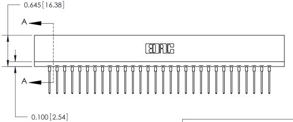
737 Series Ultra-Mate Card Edge Connector - Press Fit ACAD REFERENCE @TION - ACAD REFERENCE
