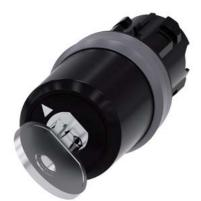
Key-operated switch BKS, 22 mm, round, plastic with metal front ring, lock number S1, with 2 keys, 2 switch positions O<I, momentary contact type, Actuating angle 45°, 10:30h/12h, key removal O, with laser labeling, inscription or symbol Customer-specific selection with SIRIUS ACT configurator (CIN)
