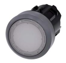
Illuminated pushbutton, 22 mm, round, plastic with metal front ring, white, pushbutton, flat, latching, Push-to-release mechanism, with laser labeling, upper case
