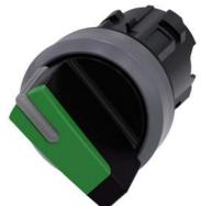
Selector switch, illuminable, 22 mm, round, plastic with metal front ring, green, selector switch, short, 2 switch positions O-I, latching, actuating angle 90°, 10:30h/13:30h, with laser labeling, inscription or symbol Customer-specific selection with SIRIUS ACT configurator (CIN)
