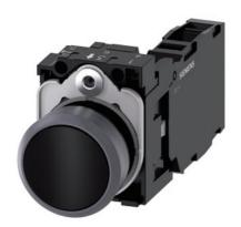
Pushbutton, 22 mm, round, plastic with metal front ring, black, pushbutton, flat, momentary contact type, with holder, 1 NO+1 NC, screw terminal, with laser labeling, symbol number according to, ISO 7000 or IEC 60417
