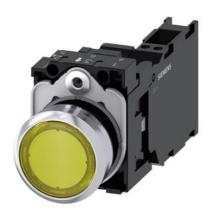
Illuminated pushbutton, 22 mm, round, metal, shiny, yellow, pushbutton, flat, momentary contact type, with holder, 1 NO+1 NC, LED module with integrated LED 110 V AC, spring-type terminal, Z=20-unit packaging
