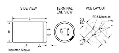
General Information Series ALC70 Dielectric Aluminum Electrolytic Description Snap-In, Aluminum Electrolytic RoHS Lead 3 Pin Short AEC-Q200 No Halogen Free Yes Component Weight 50 g Notes Dimensions D And L Include Sleeving. Shelf Life 156 Weeks
