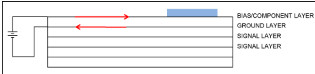
Figure 8. Better layer assignment: there are no signal layers between the bias and ground return layers.
