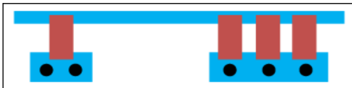
Figure 12. Using at least two grounding vias for each components reduces the effect of via parasitic inductance.
