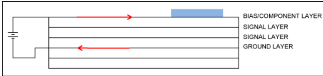
Figure 7. Incorrect layer assignment: there are signal layers between the bias layer and ground-current return path on ground layer. Bias line noise can be coupled to the signal layers.
