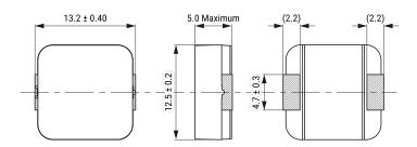
Chip Size 1250(5350) Description Surface Mount Inductor Features Power Inductors RoHS Yes Qualifications AEC-Q200 AEC-Q200 Yes Core Composite 40 (K) Temperature Rise Max. Miscellaneous
