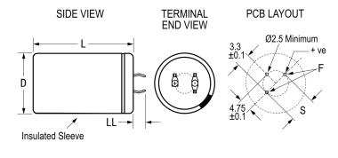
**General Information** Series PEH536 Dielectric Aluminum Electrolytic Description Snap-In, Aluminum Electrolytic RoHS Yes Lead 3 Pin Short AEC-Q200 No **Component Weight** 27 g Notes Add 0.5mm To D And 1mm To L For Sleeving. Shelf Life 208 Weeks
