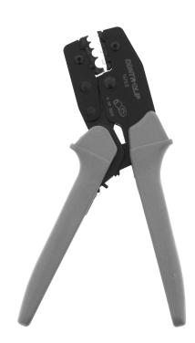
Crimping tool for non-insulated crimp lugs in ring and fork shape. Easy to use, Auto-lock for proper and complete crimping, Wire can be fed in from the side, Self-opening with built-in spring.
