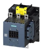
Contactor, AC-1, 275 A/690 V/40  $^\circ$ C, S6, 3-pole, 96-127 V AC/DC, F-PLC-IN with varistor, 2 NO+2 NC, Connection rail/ screw terminal
