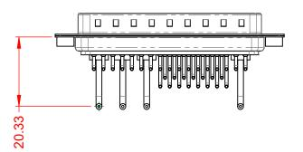
POWER/CO-AX CONTACT RATING:10A (CURRENT)(IF PRESENT)SIGNAL CONTACT CURRENT RATING:5A PER CONTACTSIGNAL CONTACT RESISTANCE: $10m\Omega$  MAX.INSULATOR RESISTANCE:5000MΩ min.DIELECTRICDIELECTRIC
