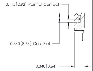
ACAD REFERENCE NO. 746 Series Ultra-Mate Card Edge Connector - Press Fit DRAWN: Part Number: 746-027-527-501 **EDAC INC** THESE DRAWINGS AND SPECIFICATIONS ARE THE PROPERTY OF EDAC INC.,AND TORONTO, ONTARIO SHALL NOT BE REPRODUCED, OR COPIED CANADA OR USED AS THE BASIS FOR THE MANUFACTURE OR SALE OF APPARATUS YOUR CONNECTION TO QUALITY & SERVICE WITHOUT WRITTEN PERMISSION.
