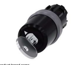
key-operated switch Siemens, 22 mm, round, plastic with metal front ring, lock no. LSG1, with 2 keys, 2 switch positions O-I, latching, actuating angle 90°, 10:30h/13:30h, key removal O+I, with laser labeling, inscription or symbol customer-specific selection with SIRIUS ACT configurator (CIN)
