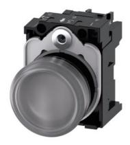
Indicator light, 22 mm, round, plastic, clear, lens, smooth, with holder, LED module, with integrated LED 24 V AC/DC, screw terminal, with laser labeling, upper case and lower case, always upper case at beginning of line
