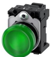
Indicator lights, 22 mm, round, Metal, shiny, green, lens, smooth, with holder, LED module with integrated LED 230 V AC, spring-type terminal, with laser labeling, upper case
