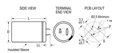
General Information Series ALC80 Dielectric Aluminum Electrolytic Description Snap-In, Aluminum Electrolytic RoHS Lead 3 Pin Short AEC-Q200 No Halogen Free Yes 60 g Component Weight Notes Dimensions D And L Include Sleeving. Shelf Life 156 Weeks
