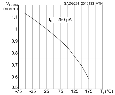
Figure 9: Normalized gate threshold voltage vs temperature
