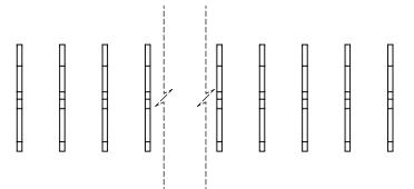
NOTE: **CONTACTS ARE HELD IN** A CARRIER FOR EASE OF ASSEMBLY
