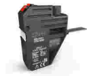
Item no.: 855-951/250-000 Current and voltage tap up to 95 mm 2 ; Primary rated current: 250 A; Secondary rated current: 1 A; Rated power: 0.2 VA; Accuracy class: 0.5; fused
