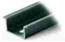
Item no.: 210-197 Steel carrier rail; 35 x 15 mm; 1.5 mm thick; 2 m long; slotted; similar to EN 60715; silver-colored
