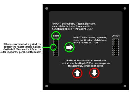
The arrangement of pins on the INPUT connector varies with matrix size and the batch in which it was produced...
