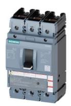
circuit breaker 3VA5 UL frame 250 breaking capacity class C 100kA @ 480 V 3-pole, line protection TM230, FTAM, In=125A overload protection Ir=125A fixed short-circuit protection Ii=5...10 x In cable connection on both sides
