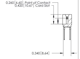
726 Series Ultra-Mate Card Edge Connector - Press Fit Part Number: 726-048-540-201 **EDAC INC** THESE DRAWINGS AND SPECIFICATIONS
