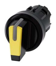
Selector switch, illuminable, 22 mm, round, plastic, yellow, selector switch, short, 3 switch positions I>O<II, momentary contact type, actuating angle  $2x45^{\circ}$ , 10:30h/12h/13:30h, with laser labeling, upper case and lower case, always upper case at beginning of line
