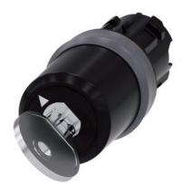
Key-operated switch BKS, 22 mm, round, plastic with metal front ring, lock No. E9 (VW), without key, 2 switch positions O-I, latching, actuating angle 90°, 10:30h/13:30h, key removal O+I, with laser labeling, upper case and lower case, always upper case at the beginning of the word
