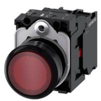
Illuminated pushbutton, 22 mm, round, plastic, red, pushbutton, flat, momentary contact type, with holder, 1NC, LED module with integrated LED 24 V AC/DC, screw terminal, with laser labeling, upper case
