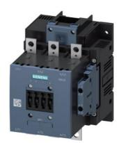
power contactor, AC-3 185 A, 90 kW / 400 V AC (50-60 Hz) / DC operation 23-26 V AC/DC auxiliary contacts 2 NO + 2 NC 3-pole, frame size S6 busbar connections drive: conventional reusable packaging = 9 units
