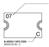
PART IDENTIFICATION: MF-MSHT020KX = 02 MF-MSHT035KX = 03MF-MSHT050KX = 05 MF-MSHT075KX = 07MF-MSHT110KX = 11 MF-MSHT125KX = 12
