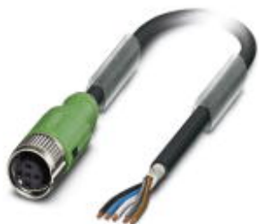
Sensor/actuator cable, 5-position, Variable cable type, shielded, free cable end, on Socket straight M12 SPEEDCON, A-coded, cable length: Free input (0.2 ... 40.0 m)
