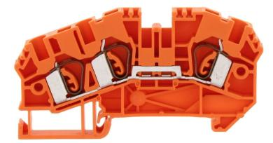
Feed-through terminal, Tension-spring connection, Mounting type: Mounting rail TS 35/7.5, Rated cross-section: 4 mm<sup>2</sup>, Width: 6.1 mm, Colour: Orange
