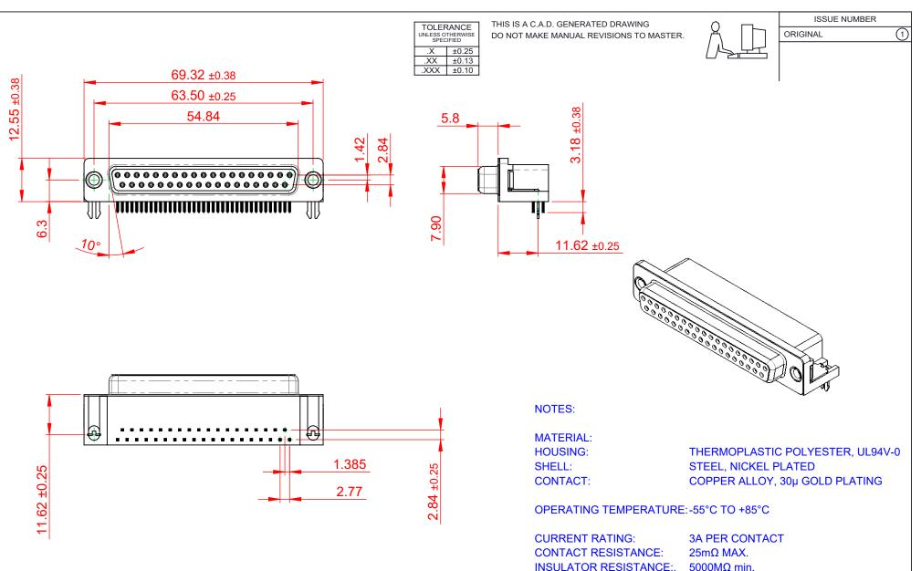
DIELECTRIC WITHSTANDING VOLTAGE: 1000V AC rms
