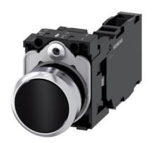
Pushbutton, 22 mm, round, metal, shiny, black, pushbutton, flat, momentary contact type, 1 NO+1 NC, screw terminal, with laser labeling, upper case
