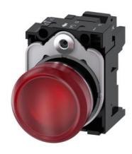
Indicator lights, 22 mm, round, metal, shiny, red, lens, smooth, with holder, LED module with integrated LED 110 V AC, spring-type terminal, Z=20-unit packaging
