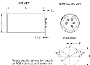
Series ALF70 Dielectric Aluminum Electrolytic Style Press-Fit Description Press-Fit, Aluminum Electrolytic RoHS Yes Lead 5 Pin Press-Fit AEC-Q200 No Halogen Free Yes **Component Weight** 125 g Dimensions D And L Include Sleeving. Notes Shelf Life 156 Weeks
