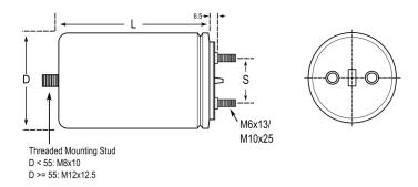
General Information Series C44A Dielectric Metallized Polypropylene Style Can RoHS With Exemptions **REACH** SVHC (Pb - CAS 7439-92-1) cc1c1ec4-db9e-4815-b26b-e8a34ddfb776 SCIP Number Lead Threaded Studs M6 AEC-Q200 No Component Weight 375 g Thermal Resistance = 2 C/W. Miscellaneous
