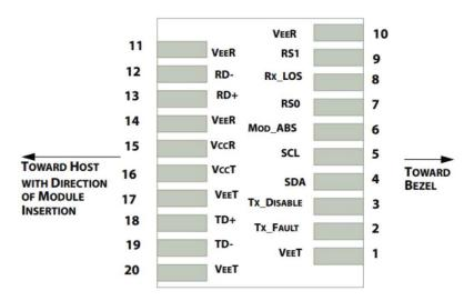
**Electrical Pin-out Details for SFP**
