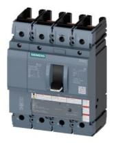
circuit breaker 3VA5 UL frame 250 breaking capacity class M 35kA @ 480V 4-pole, line protection TM230, FTAM, In=250A overload protection Ir=250A fixed short-circuit protection Ii=5...10 x In N conductor protection 100% without connection
