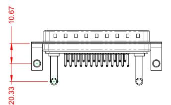
**OPERATING TEMPERATURE:** -55°C ~ 125°C 40A (CURRENT) POWER/CO-AX CONTACT RATING: (IF PRESENT) SIGNAL CONTACT CURRENT RATING: 5A PER CONTACT SIGNAL CONTACT RESISTANCE:  $10m\Omega$  MAX. **INSULATOR RESISTANCE:** 5000MΩ min.
