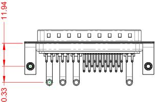
POWER/CO-AX CONTACT RATING: 30A (CURRENT) (IF PRESENT) SIGNAL CONTACT CURRENT RATING: 5A PER CONTACT SIGNAL CONTACT RESISTANCE:  $10m\Omega$  MAX. **INSULATOR RESISTANCE:** 5000MΩ min.
