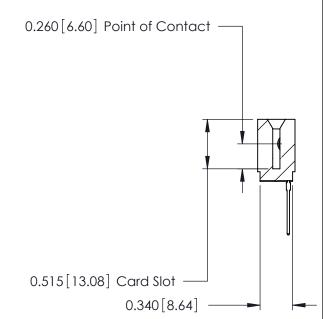
ACAD REFERENCE NO. 746-ENG MASTER 746 Series Ultra-Mate Card Edge Connector - Press Fit DRAWN: J.LEE DATE: AUG 20/09 Part Number: 746-026-540-101 CHECKED: DATE: **EDAC INC** SCALE: SHEET 1 OF 1 THESE DRAWINGS AND SPECIFICATIONS ARE THE PROPERTY OF EDAC INC., AND TORONTO, ONTARIO SHALL NOT BE REPRODUCED, OR COPIED DRAWING NUMBER CANADA OR USED AS THE BASIS FOR THE 746-ENG MASTER MANUFACTURE OR SALE OF APPARATUS YOUR CONNECTION TO QUALITY & SERVICE WITHOUT WRITTEN PERMISSION.
